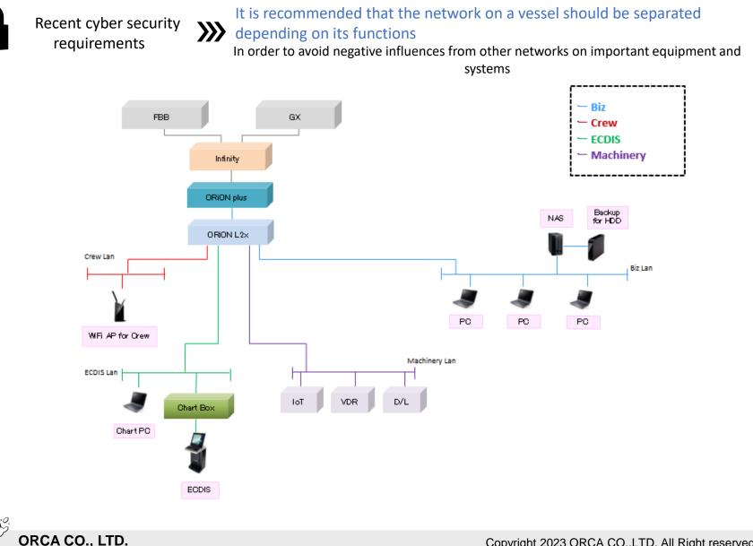
Copyright 2023 ORCA CO., LTD. All Right reserved. 1 Explanation of VLAN configuration on a vessel using OL2x
